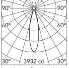
Luminous flux luminaire 958 lm
