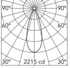
Luminous flux luminaire 956 lm
