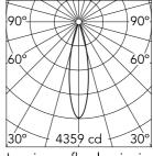
Luminous flux luminaire 933 lm
