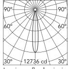
Luminous flux luminaire 1058 lm
