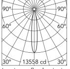
Luminous flux luminaire 1395 lm (EXTREME CUT OFF)
