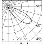
Luminous flux luminaire 482 lm
