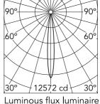
Beam Angle: 11° h(m) = E(Ix)D(m) 12572 0.20 3143 0.40 3 1397 0.60 4 786 0.80 5 503 1.00
