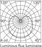
Luminous flux luminaire 508 lm
