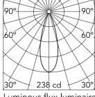
Luminous flux luminaire 77 lm
