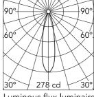
Luminous flux luminaire 70 lm
