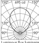
Luminous flux luminaire 1624 lm
