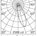
Luminous flux luminaire 1909 lm (EXTREME CUT OFF)
