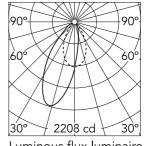
Luminous flux luminaire 1918 lm (EXTREME CUT OFF)
