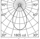
Luminous flux luminaire 1799 lm (EXTREME CUT OFF)
