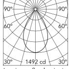
Luminous flux luminaire 1487 lm (EXTREME CUT OFF)
