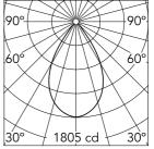
Luminous flux luminaire 1799 lm (EXTREME CUT OFF)
