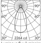
Luminous flux luminaire 1576 lm (EXTREME CUT OFF)
