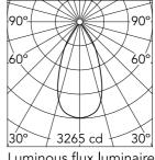
Luminous flux luminaire 2270 lm (EXTREME CUT OFF)
