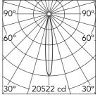
Luminous flux luminaire 1698 lm (EXTREME CUT OFF)
