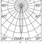
Luminous flux luminaire 2208 lm (EXTREME CUT OFF)
