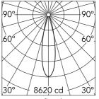
Luminous flux luminaire 1743 lm (EXTREME CUT OFF)
