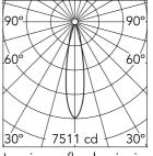
Luminous flux luminaire 1367 lm (EXTREME CUT OFF)
