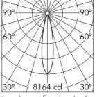
Luminous flux luminaire 1486 lm (EXTREME CUT OFF)
