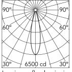
Luminous flux luminaire 1297 lm (EXTREME CUT OFF)
