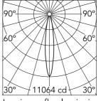
Luminous flux luminaire 1363 lm (EXTREME CUT OFF)
