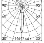
Luminous flux luminaire 1871 lm (EXTREME CUT OFF)
