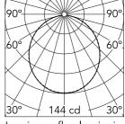
Luminous flux luminaire 405 lm
