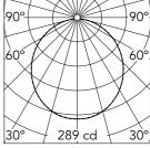
Luminous flux luminaire 809 lm
