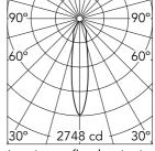
Luminous flux luminaire 734 lm
