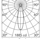
Luminous flux luminaire 700 lm
