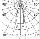
Luminous flux luminaire 322 lm (EXTREME CUT OFF)
