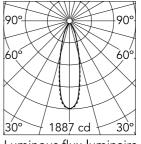
Luminous flux luminaire 537 lm (EXTREME CUT OFF)
