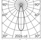
Luminous flux luminaire 576 lm (EXTREME CUT OFF)
