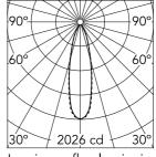
Luminous flux luminaire 576 lm (EXTREME CUT OFF)
