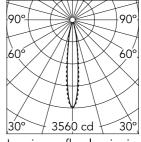
Luminous flux luminaire 360 lm (EXTREME CUT OFF)
