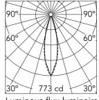
Luminous flux luminaire 167 lm (EXTREME CUT OFF)
