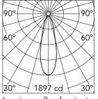
Luminous flux luminaire 558 lm (EXTREME CUT OFF)
