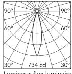
Luminous flux luminaire 138 lm (EXTREME CUT OFF)
