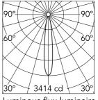
Luminous flux luminaire 377 lm (EXTREME CUT OFF)
