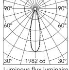
Luminous flux luminaire 540 lm (EXTREME CUT OFF)
