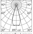
Luminous flux luminaire 281 lm (EXTREME CUT OFF)
