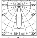
Luminous flux luminaire 445 lm (EXTREME CUT OFF)
