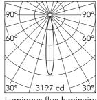
Luminous flux luminaire 297 lm (EXTREME CUT OFF)
