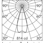
Luminous flux luminaire 248 lm (EXTREME CUT OFF)
