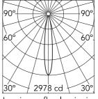
Luminous flux luminaire 277 lm (EXTREME CUT OFF)
