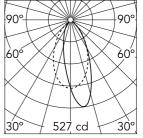
Luminous flux luminaire 407 lm (EXTREME CUT OFF)
