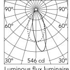
Luminous flux luminaire 421 lm (EXTREME CUT OFF)
