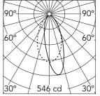
Luminous flux luminaire (EXTREME CUT OFF) 421 lm
