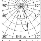
Luminous flux luminaire 529 lm (EXTREME CUT OFF)
