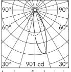
Luminous flux luminaire 577 lm (EXTREME CUT OFF)
